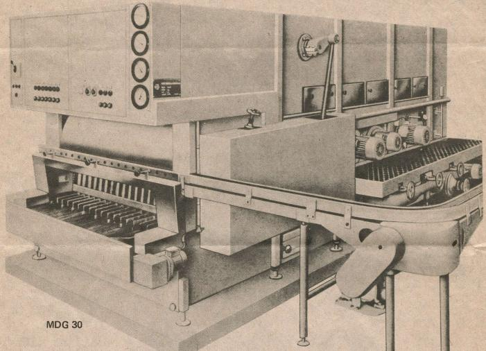
HVN 24/KRN 8 vacuum filling and crown sealing machine. Capacity: Up to 14000 bottles per hour. Other capacities available.
